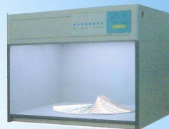
P60(6) (TILO, China) 6 light sources, 710 x 530 x 620 mm
