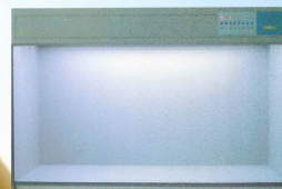
P120 (TILO, China) 8 light sources, 1310 x 600 x 800 mm
