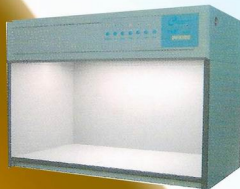
T60(5) (TILO, China) 5 light sources, 710 x 405 x 570 mm
