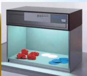
CAC60 (VeriVide, UK) 4 light sources, 710 x 420 x 570 mm
