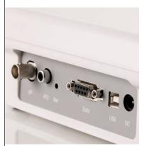
The FiveEasy Plus series meters allows data to be exported either directly to a printer or a PC for further processing using its RS232 or USB ports.
